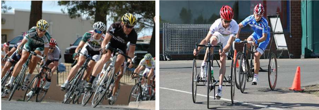
Able-bodied athletes countering turning forces on bikes and a trike. While the bikers counter centrifugal forces by leaning the body and machine at a uniform angle, the trike rider can do so only by separating his body angle from that of the trike.
